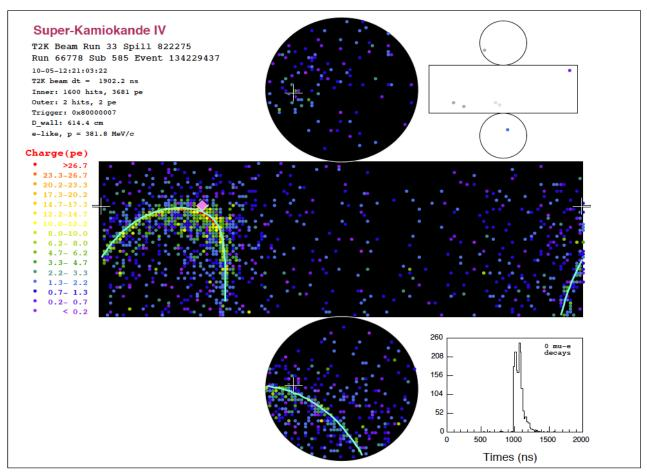
In this projected diagram of cylinder-shaped Super-Kamiokande, each colored dot shows a photomultiplier that detected light (these photomultipliers are mounted on the inside wall of the detector). Electron neutrinos interact with water in the detector to produce electrons, which subsequently induce electromagnetic showers to eventually emit Cherenkov light that is detected in a ring-shaped structure.
